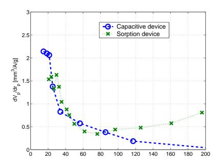
Figure 10: Comparison between pore radius distribution from thermoporometry using CS and from sorption isotherm using SD for W/C=0.4 cement paste.
