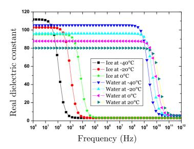
Figure 1: Frequency dispersion of water and ice real dielectric constants at different temperatures.
