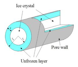
Figure 12: Schematic representation of an elementary cylindrical pore.
