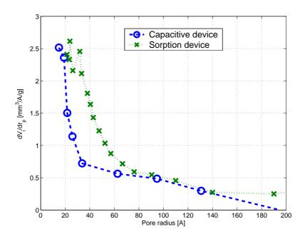
Figure 11: Comparison between pore radius distribution from thermoporometry using CS and from sorption isotherm using SD for W/C=0.5 cement paste.
