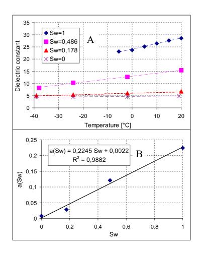
Figure 6: Evolution of the apparent dielectric constant and its derivation with temperature at a fixed saturation ratio for cement paste P5-1d.
