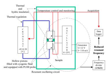
Figure 2: Schematic diagram of the capacitive sensor-based apparatus. The oscillator was implementing a frequency divider in order to reach a low frequency range (in the order of several kHz) before outputting the resonant frequency to the data logger device. Galden PFPE HT200 from Solvay Solexis company is used as cryogenic fluid for its low static dielectric constant (about 2 at  $20~^{0}$ C).
