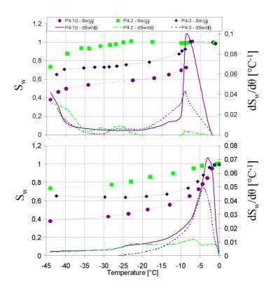
Figure 8: Freezing (upper graph) and thawing (lower graph) of W/C=0.4 cement paste submitted to different curing conditions.
