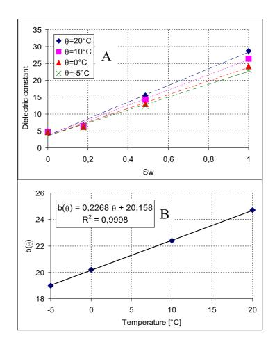
Figure 7: Evolution of the apparent dielectric constant and its derivation with saturation at a fixed temperature for cement paste P5-1d.
