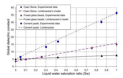
Figure 5: Comparison between measured and calculated dielectric constants of a non-saturated porous medium. The calculation is made using the three-phase Lichtenecker model with  $\alpha = \phi$  in (6), thus leading to (7).
