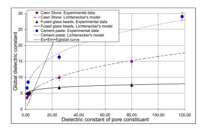
Figure 4: Comparison between measured and calculated dielectric constants of a fully saturated porous medium. The calculation is made using the two-phase Lichtenecker model with (4) or (6) in which  $\varepsilon_w = \varepsilon_f$  and  $S_w = 1$ .
