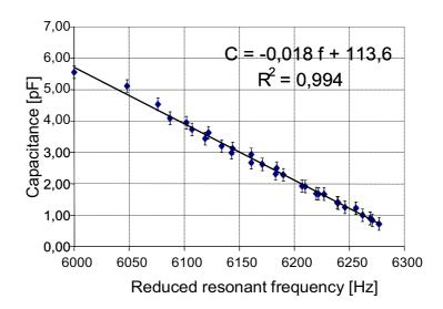
Figure 3: Sample-electrode capacitance versus measured reduced resonant frequency.
