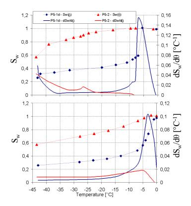
Figure 9: Freezing (upper graph) and thawing (lower graph) of W/C=0.5 cement paste submitted to different curing conditions.
